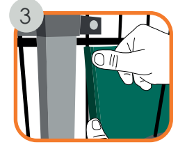
3 Attach PVC strip with a holder to the beginning or end of the fence
